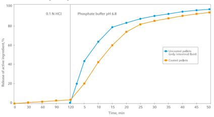
The release of the active ingredient was tested using the coated pellets by placing them in 0.1 N HCl for a period of 2 hours and afterwards in phosphate buffer (pH 6.8). Pellets coated with AquaPolish® E based on methacrylic acid-ethyl acrylate copolymer type B.
