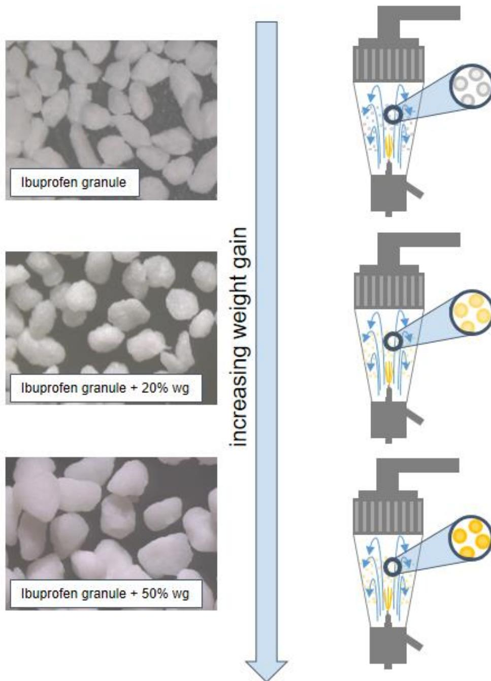
**Figure 4:** Flow chart of gradual application of HMC onto Ibuprofen granules
