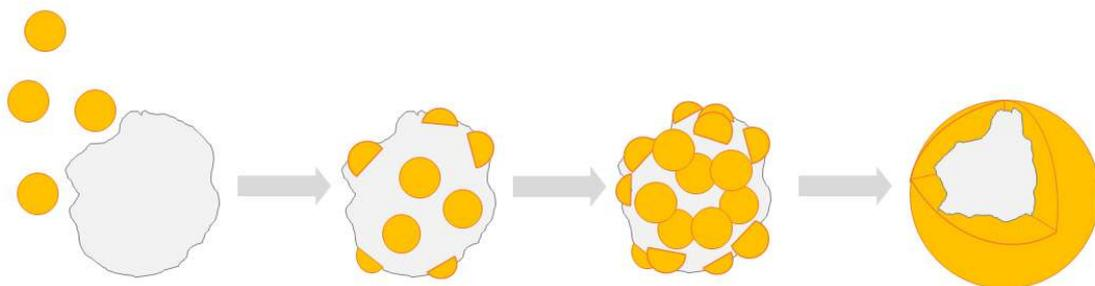
**Figure 2:** Stepwise formation of a HMC onto solid particles using BonuWax®
