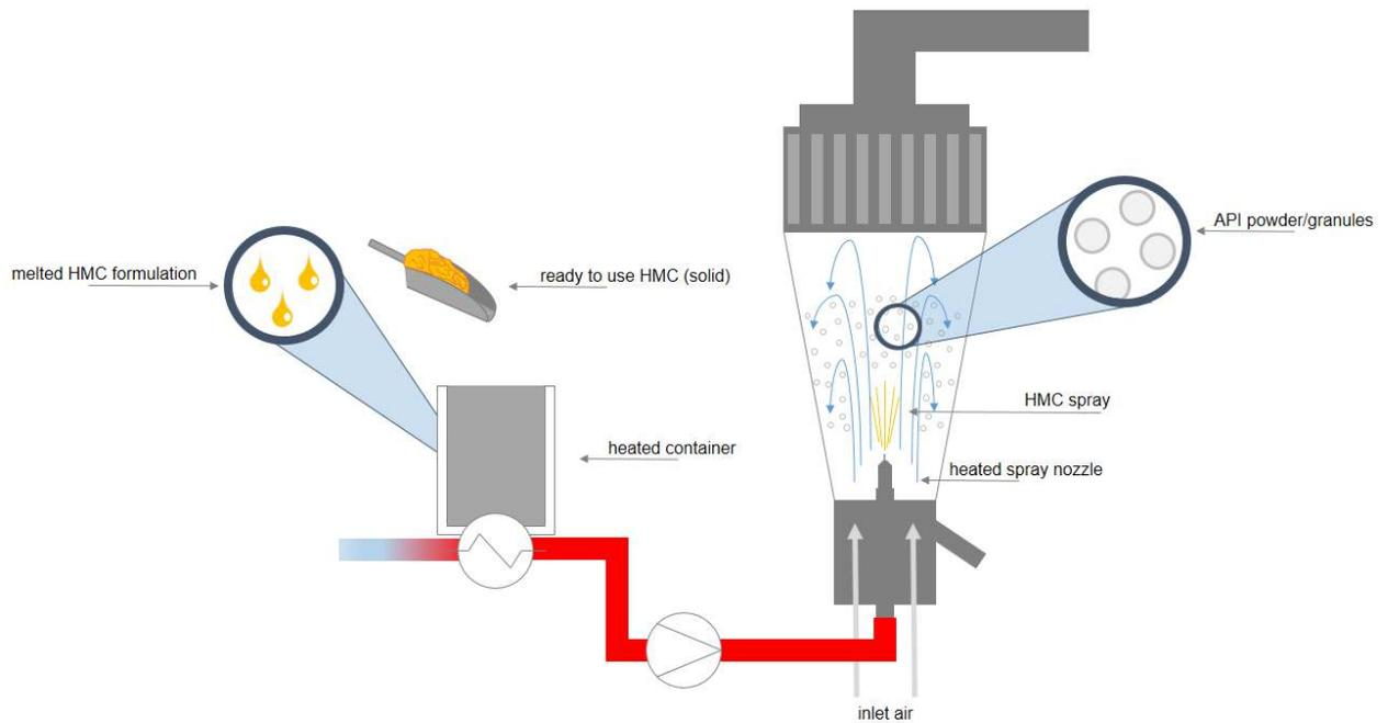
**Figure 1:** General Process of HMC using fluidized bed technology
