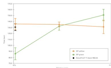
Figure 3: The drying time of the BP yellow (orange line) and BP green (green line) at each dilution level and the drying time of the BonuPrint<sup>®</sup> F black 980.04 (black point) as reference. The drying time of the BP yellow remained nearly constant due to the strong intermolecular force of water whereas, the drying time of BP green was increased due to intermolecular force of thinner solution.
