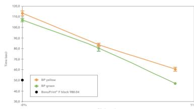
Figure 2: The viscosity of the BP yellow (orange line) and BP green (green line) at each dilution level and the viscosity of the BonuPrint<sup>®</sup> F black 980.04 (black point) as reference. The viscosity of both BPs were reduced due to addition of thinner solution.
